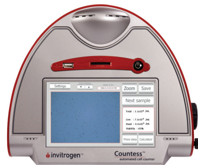
Figure 1. The Countess ® Automated Cell Counter. The cell counter was used as the standard automated cell counter for these experiments. The Countess ® cell counter uses the trypan blue exclusion method to calculate cell concentration and provide viability information.
