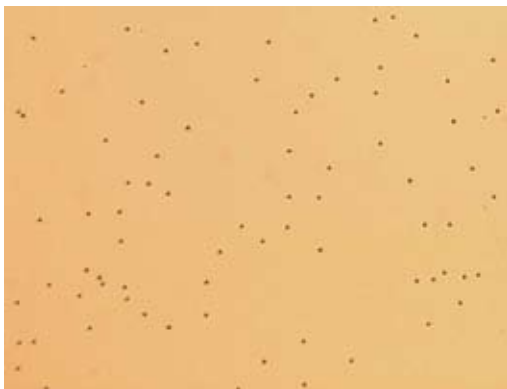
Figure 4—Red blood cells read on the Countess™ Automated Cell Counter are counted as beads, and will not give a viability reading.
