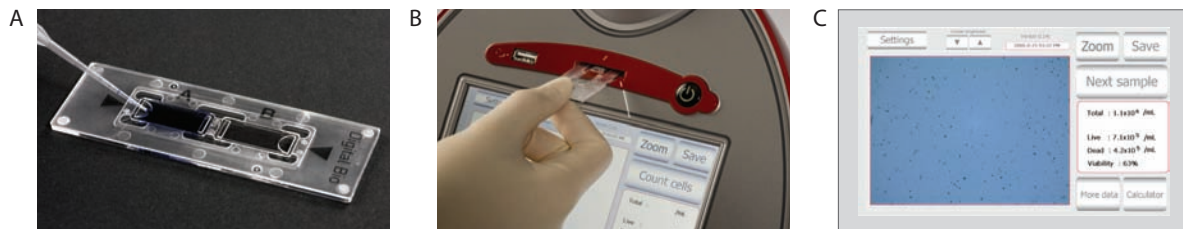
Figure 2. Countess™ Automated Cell Counter. The Countess™ Automated Cell Counter eliminates the tedium and subjectivity of manual cell counting. Automated counting frees up your time, reduces eyestrain, and minimizes subjective judgments that can lead to error. It takes 3 simple steps: (A) Mix 10 \mu L of sample with 10 \mu L of trypan blue, and pipet into a Countess™ Chamber Slide. (B) Insert slide into the instrument. (C) Press the "Count cells" button, and results are displayed in 30 seconds.
