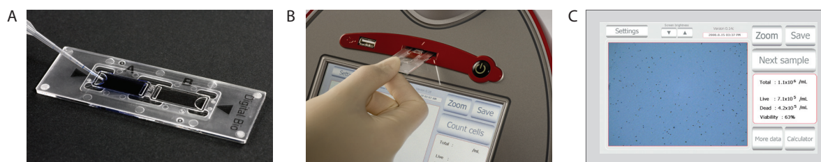
Figure 1—Countess™ Automated Cell Counter. The Countess™ Automated Cell Counter eliminates the tedium and subjectivity of manual cell counting. Automated counting frees up your time, reduces eye strain, and minimizes subjective judgments that can lead to error. It takes 3 simple steps: (A) Mix 10 \mu L of sample with 10 \mu L of trypan blue, and pipet into Countess™ chamber slide. (B) Insert slide into the instrument. (C) Press the “Count cells” button, and results are displayed in 30 seconds.
